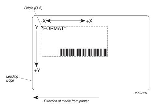
**Default X and Y origins:** This illustration shows the default X and Y origins. You can control the default X origin (top of form) with PrintSet or with the Test and Service DIP switches. You can control the default Y origin with the DIP switches only.
